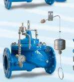
Valves for minimum-maximum level control XLC 340 and 440 or constant (proportional) level control XLC 360 and 460 For regulation of water level in tanks by means of pilots with float connected to the circuit of the valve.
