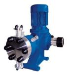
Liquid end: AISI 316L ; PP ; PVDF Flow-rate adjustment: Manual or automatic by AKTUA Pressure up to124 bar Flow rate up to 660 L/h API 675 Standards - CE and ATEX marking
