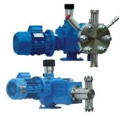
Liquid end: SS 316L, PP, PVDF, different material on request Flow-rate adjustment:manual, electrical 4÷20 mA, Pneumatic 3-15 psig and/or SMART (protocol HART) servomotor and/or by frequency converter drivers Multiple head execution with different mechanism size and gear ratio Pressure up to 350 bar Flow rate up to 8,000 l/h (single head)
