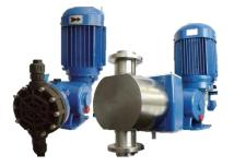
Liquid end: SS 316 L or PVC Flow-rate adjustment: manual, electrical 4÷20 mA Pressure up to 10 bar (higher on request) Flow rate up to 1,000 l/h
