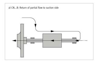
Figure 3a: The carrying of the Partial Flow of various types
