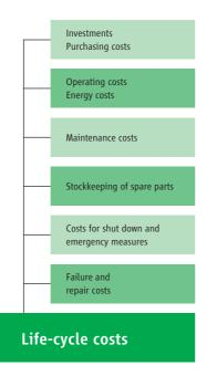
Figure 1: Life-cycle costs of centrifugal pump
