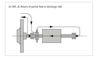
Figure 3b: The carrying of the Partial Flow of various types
