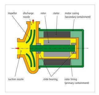
Figure 2: Simplified diagram of a canned motor pump
