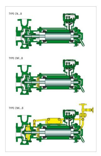
Figure 5: Modular construction principle
