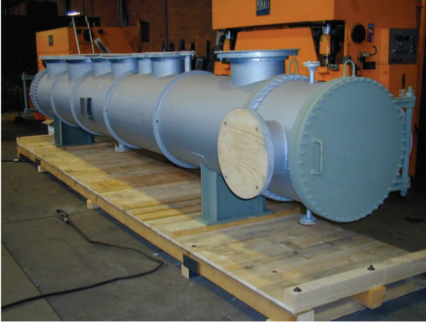
Qatar Application Desalination Plant Vacuum system Precondenser
