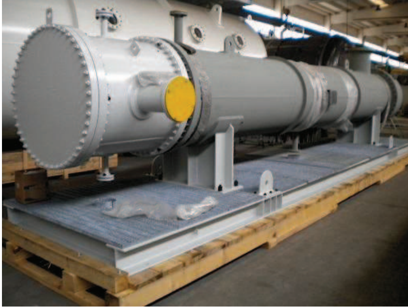
Italy Application Refinery Plant VDU Vacuum system Precondenser
