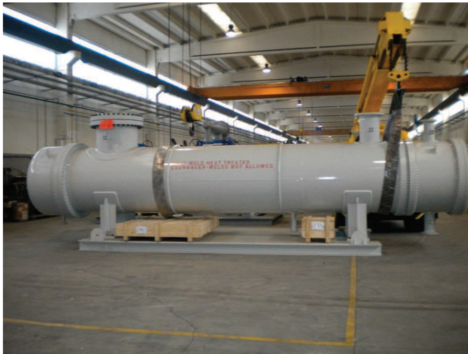
Portugal Application Refinery Plant VDU Hybrid Vacuum system - Precondenser
