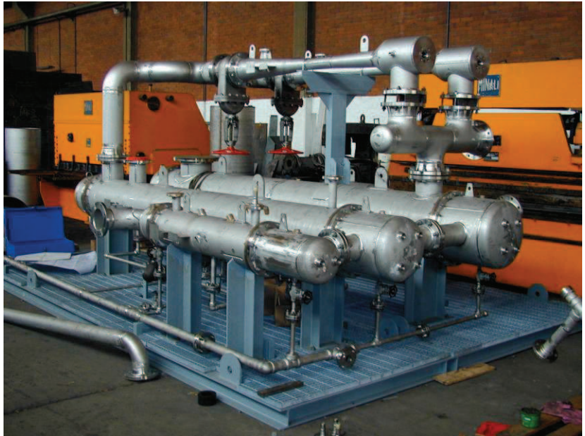
Saudi Arabia Application Desalination Plant Vacuum system
