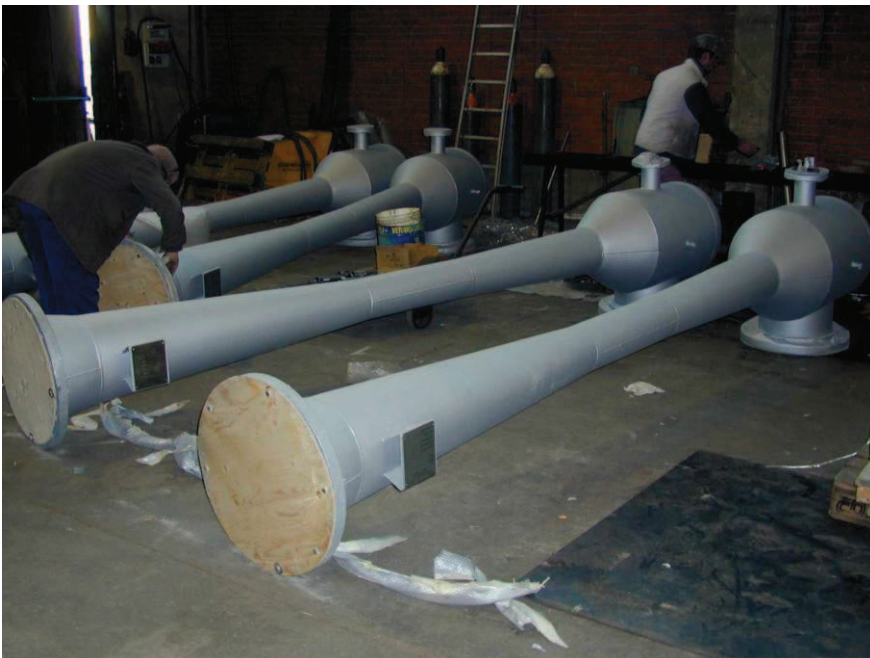
Qatar Application Desalination Plant Vacuum system 1 st stage ejector
