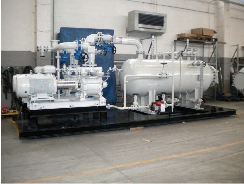
Portugal Application Refinery Plant VDU Hybrid Vacuum system - 3 rd stage LRP with gas separator
