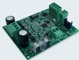
Scheda Controllo motori brushless – Electronic control board for brushless motors
